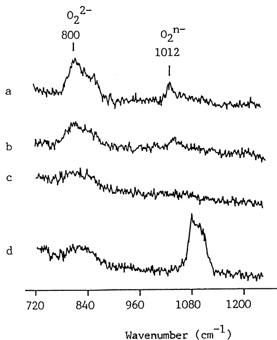
FIG. 7. Raman spectra obtained when a 10 mol% BaCO 3 /LaOBr catalyst was under (a) O 2 at 100°C, (b) O 2 at 300°C, (c) O 2 at 650°C, and (d) CH 4 :O 2 (2.6:1) at 650°C.
